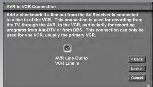
Figure 1. AVR to VCR Connection screen.
